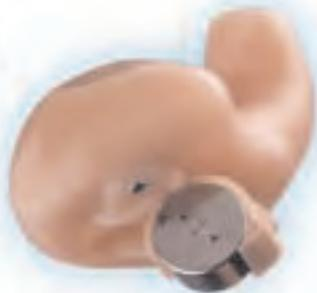
Your Libra ITE is “on” anytime a functioning battery is properly placed in the compartment, and the battery door is closed.
