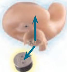
Remove the existing battery either by pushing it out the top of the door, or pulling it straight out.
