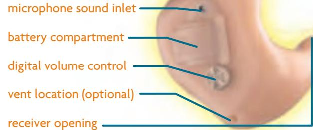
Your Libra CE Digital In-The-Ear (ITE) has been custom-made with the precise electronic circuitry controls to match your particular hearing requirements.
