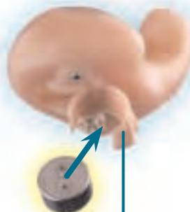
Close the battery compartment by swinging the door until it snaps securely. NEVER FORCE THE DOOR SHUT. This could result in serious damage. If the door will not close securely, check that the battery is placed properly in the compartment.
