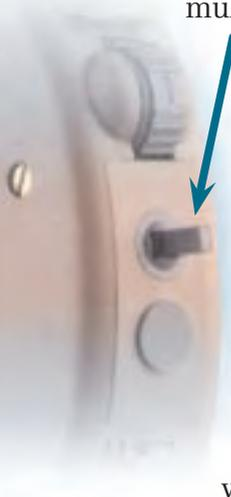
Libra BTEs with a horizontal multimemory switch let you choose between two settings to compensate for different listening environments. When the switch is towards the left, your instrument is most likely programmed for normal listening situations like one-to-one conversations.
