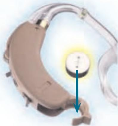
Close the battery compartment by swinging the door until it snaps securely. NEVER FORCE THE DOOR SHUT. This could result in serious damage. If the door will not close securely, check that the battery is placed properly in the compartment.
