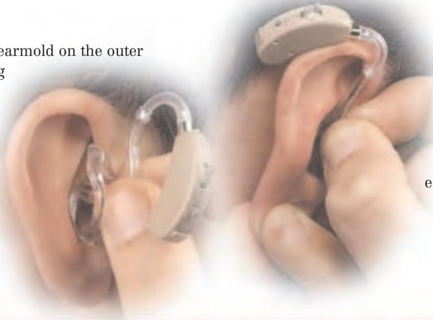
Carefully place the instrument behind your ear with the earhook and earmold tubing wrapped over the top.
