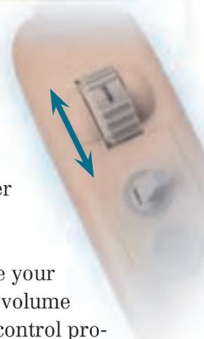
The volume control enables you to adjust the amount of amplification provided by the instrument. You may wish to change levels as you encounter different listening situations.
