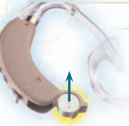
Remove the existing battery by pushing it out the top of the door.
